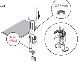
8 Screw the supply hoses on the angle valves.
